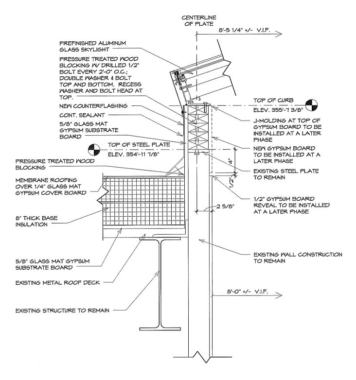
NOTE: SKYLIGHT SLOPE TO BE 4:12. APPLIES TO ALL SIDES OF SKYLIGHT. SEE DETAIL RD-21 FOR DIMENSIONS OF SKYLIGHT.
